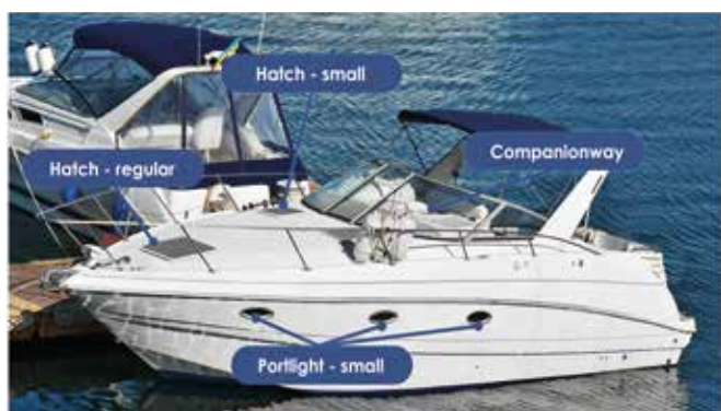
Hatches – Small inside max 300 x 300 mm (12" x 12")
