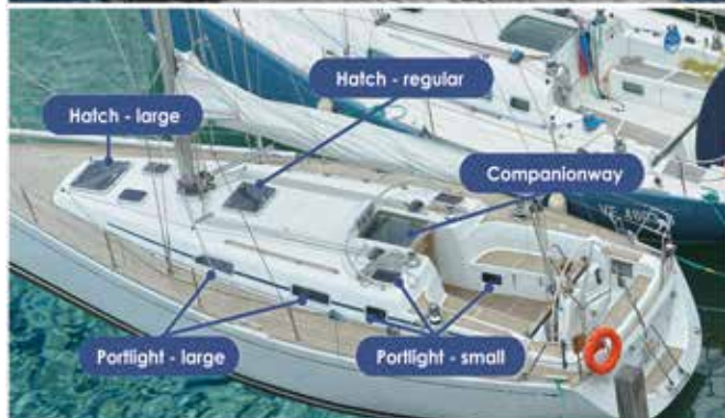
Hatches – Regular inside max 520 x 520 mm (21" x 21")
